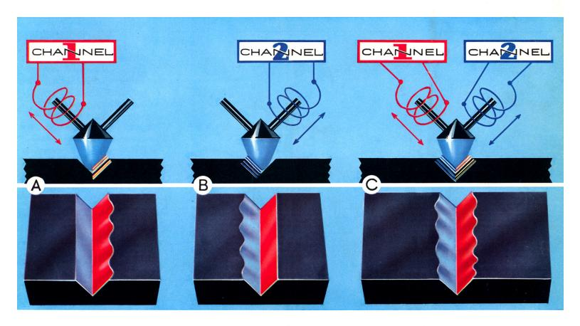
With the stereophonic record different sounds are recorded on each side of the record groove. To capture the fullness, depth and fidelity that is on the record the reproducing system must parallel the recording system. The Seeburg Two-Channel Stereo System does this superbly—from the pickup through the amplifiers, to the speakers.
