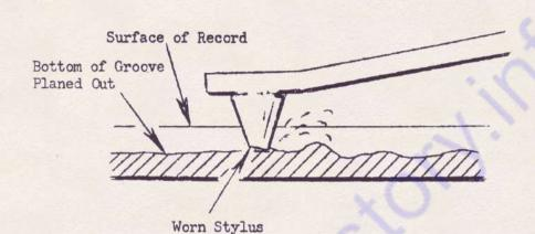
For this reason, we supply a long wearing diamond stylus in our stereo pickup and recommend that replacement styli have diamond tips. If sapphire styli are used for stereo machines, they should be replaced much more frequently than on monaural machines.
